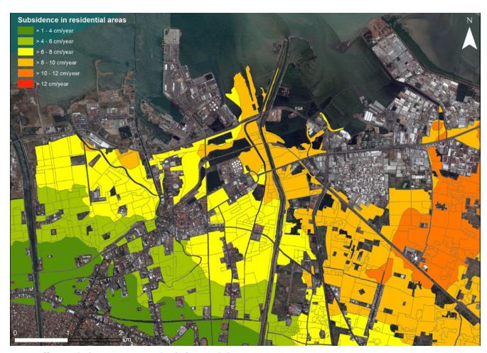
FIGURE 22: Terrain and infrastructure motion product for Semarang, Indonesia (Credit: JR. Satellite imagery: Pleiades © (2015) CNES, Distribution Airbus DS)
